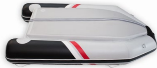
Inflatable V-shaped hull
