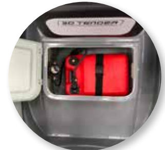
Fuel tank integrated into console
