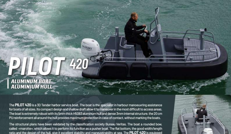
In order to secure the boat, handrails are present all around the **PILOT 420**. This boat is self-draining.On request, the shell of the Pilot 420 can be declined in other colors, and the fenders in white
