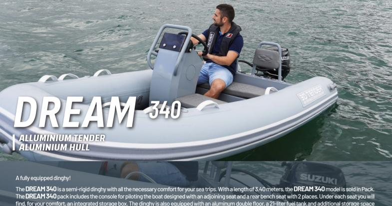
find, for your comfort, an integrated storage box. The dinghy is also equipped with an aluminum double floor, a 21-liter fuel tank and additional storage space in the bow. The double floor of the DREAM 340 allows water to drain from the bottom of the hull. Its flat deck is covered with a non-slip EVA foam.
