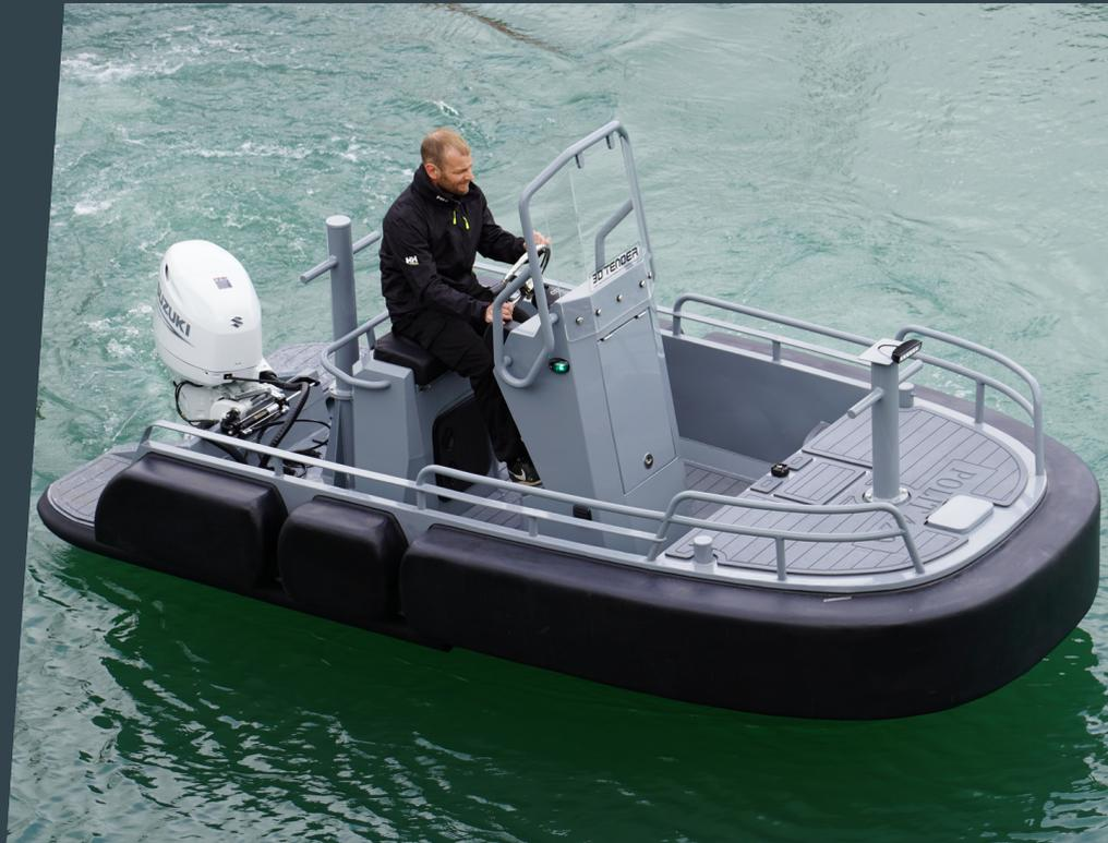
The rounded bow allows it to perform its function as a pusher boat. The flat bottom, the good width/length ratio and the design of the hull, give it excellent stability and maneuverability at sea.
